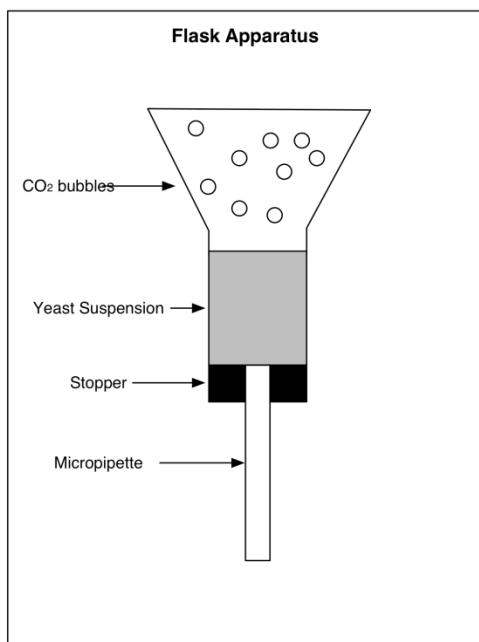
The data shown below were collected at regular time intervals to assess the amount of suspension (mL) pushed in the glass tube due to CO<sub>2</sub> accumulation
